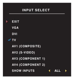
**VGA** — Select when your TV display is being used as a computer monitor and you have connected the computer using a VGA cable. See "Bottom View" on page 8 for the location of the VGA connector.
